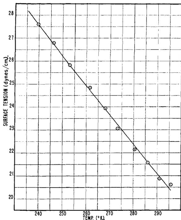
Fig. 2.—Borazole surface tension.
